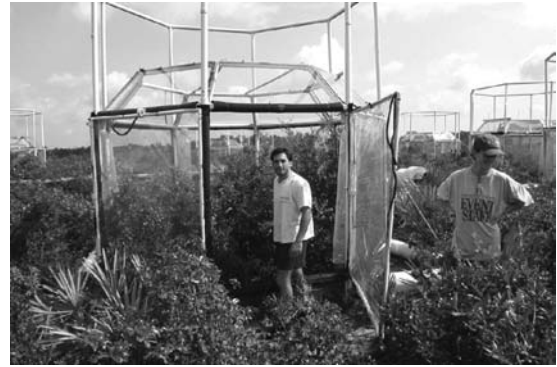
Figure 3.30 Open-top chambers at the Kennedy Space Center (Florida, USA) used to manipulate levels of atmospheric carbon dioxide. (Courtesy Peter Stiling.)
