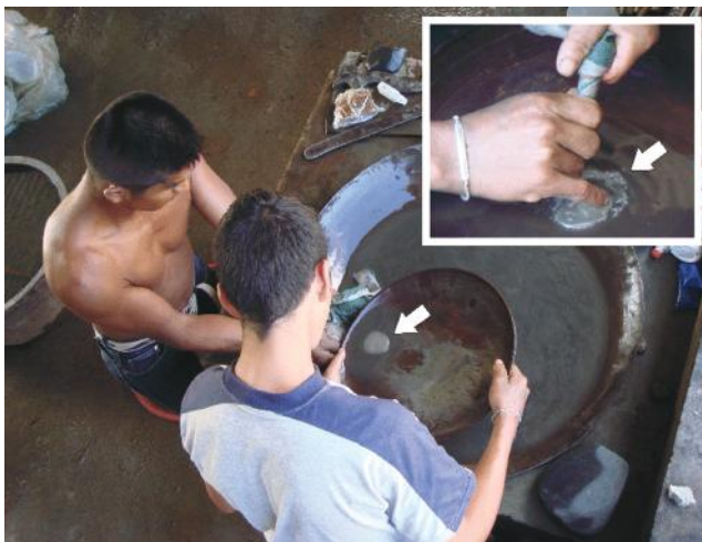
Figure 1.5 Mercury being used to extract gold from ore mined in Portovelo, Ecuador (June 2007). Pulverized ore is agitated with a puddle of mercury (arrows) to form a gold–mercury amalgam, which in this picture, is being placed into a piece of cloth. Mercury is hand-squeezed from the amalgam and remaining mercury is driven off by heating with a propane torch. This process results in substantial human exposure and mercury release into the environment. (Note that the person wringing the mercury from the amalgam has a silver bracelet into which the mercury will also readily dissolve to form a silver–mercury amalgam.) (Courtesy of Lane, K., College of William & Mary.)
