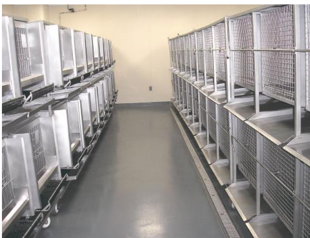
Figure 9.2 An avian toxicity testing facility in which a series of doses are fed to subsets of mallard ducks so that lethal or nonlethal effects can be quantified.
