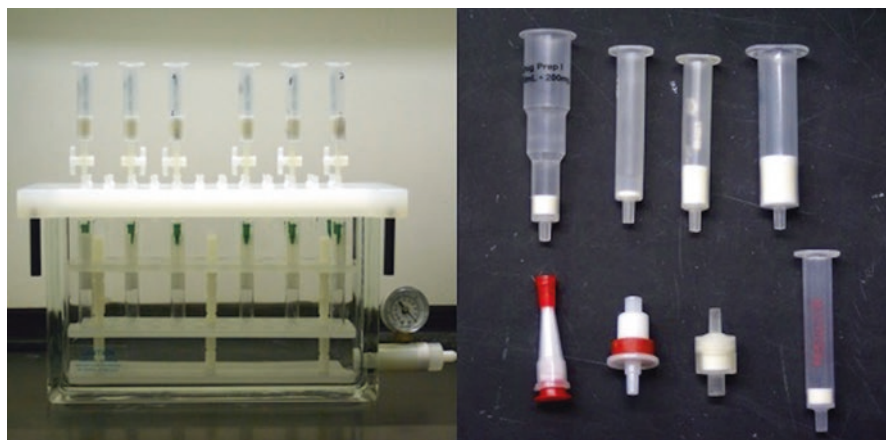
Fig. 13.8 Solid-phase extraction apparatus and a variety of column types used in the preprocessing of samples in metabolomics experiments. (Image courtesy: Jeff Dahl shared through Wikipedia Commons by CC BY-SA 3.0 license)
